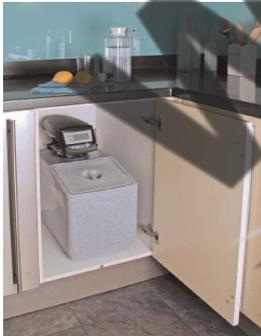
Point of Entry ion exchange systems consist of a vessel through which the water flows, down through the ion exchange media where the nitrate is held. These systems are big enough to treat the water for the whole house (treating the drinking water, bathroom water, hot water, dishwasher water etc). The systems have automatic regeneration with salt so are always ready for use. These Point of Entry systems fit under the sink or in a utility rooms.
