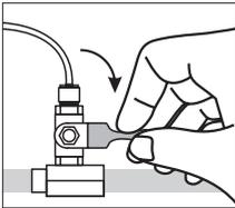
Turn on the mini valve of the water supply as shown in the figure.
